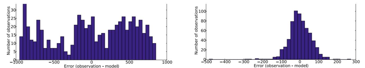
**Figure 3.** Histogram of distances from observed data to expected "true data", when cleansing either raw data (left) or preprocessed data where cycles are subtracted (right). The distribution takes on a Gaussian shape after preprocessing.
