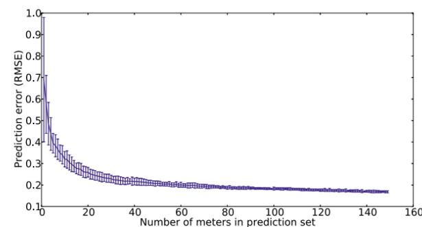
Figure 2. Forecast error (mean and standard deviation) as a function of the number of meters accumulated in the forecasted time series.
