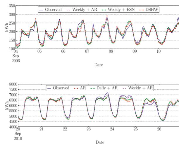
Figure 5. Sample forecasts made by some of the forecasting models under study. Distribution substation data on top, transmission network data on bottom.
