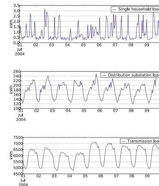
Figure 1. Sample time series of power load data at end user, distribution substation, and transmission level.
