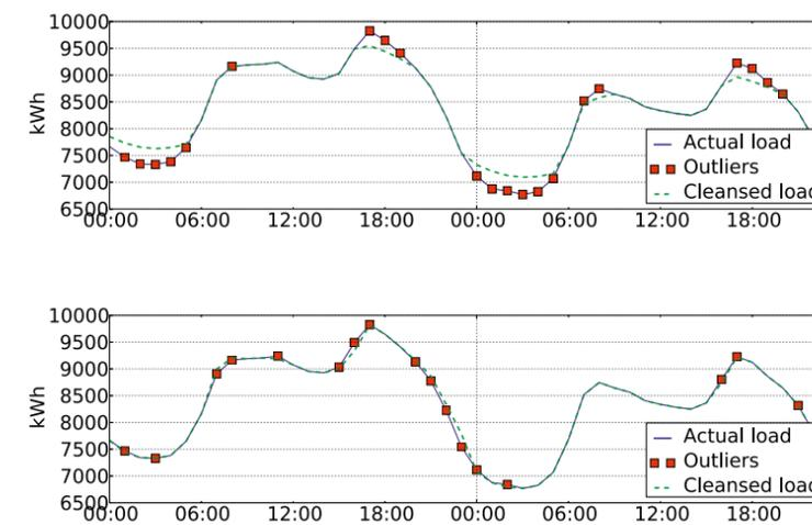
Figure 4. Examples of cleansed load data, using the original algorithm (top) and after subtracting cycles (bottom). The original algorithm has a higher tendency to cut peaks and fill troughs.
